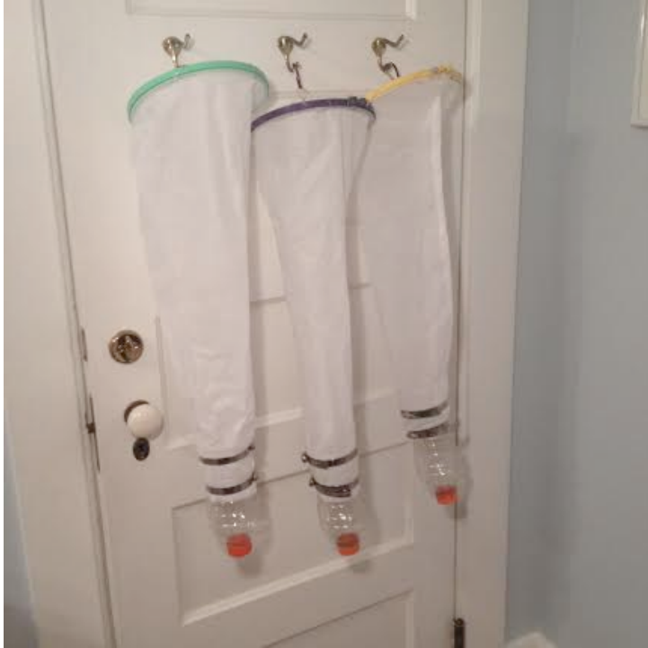
Figure 4. Plankton nets developed by student researchers from the Poughkeepsie Day School were distributed to citizen science volunteers to help with monitoring the spread and population dynamics of BRS. The nets were constructed with lightweight materials that could commonly be purchased at local stores for less than $10. Photo credit: Julia Roellke
